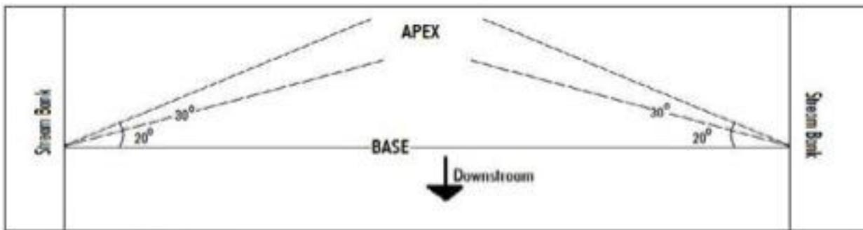
**Figure 1:** Vortex Rock Weir design
