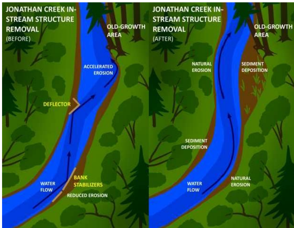
Figure 1. Bank stabilizer (JC-L04) and wing deflector (JC-L05) causing accelerated erosion into an old-growth area downstream before removal (left) and predicted flow after structure removal (right).
