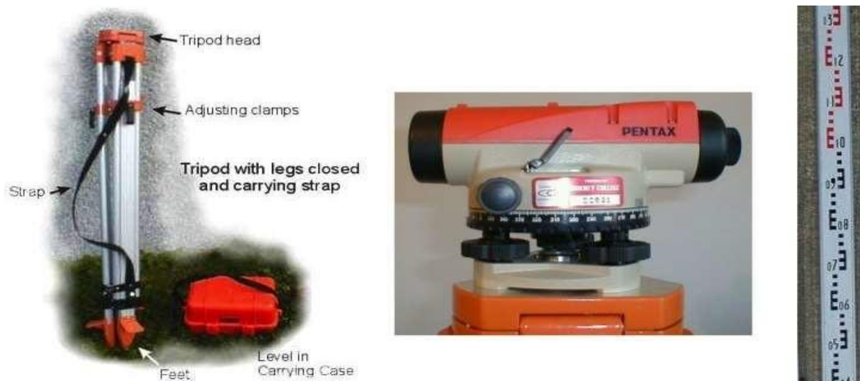
Figure 8: Pictures of the 3 pieces of equipment required for surveying: the tripod (left), the automatic level (center) and the staff (right) (Photographs of surveying equipment, n.d.).
