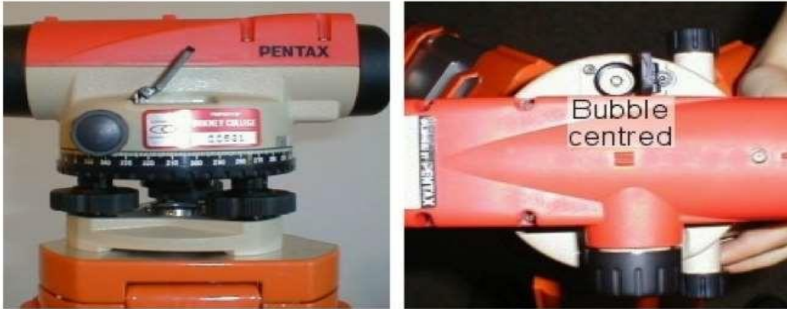
Figure 9: The automatic level must be secured onto the tripod head (left) before using the 3 leveling screws to bring the bubble within the circle on the spherical level (right). Once the bubble is centered, staff readings can be taken (Photographs of surveying equipment, n.d.).
